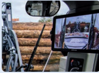
Multi-view front camera system for large attachments
