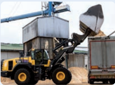
High-dump and light material buckets
