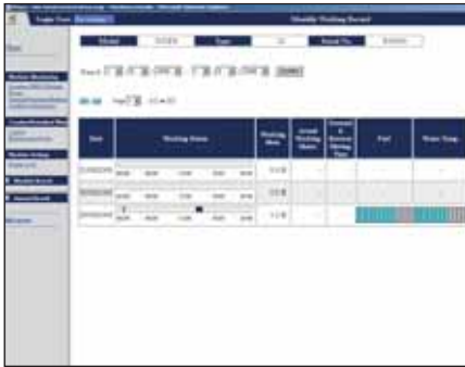
Machine working time - With the “daily working record” chart, get precise engine running time data: when your machine was started and when it was shut down, as well as total engine running time.
