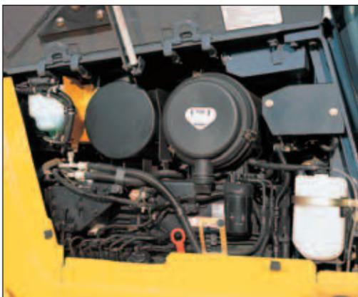
A radiator coolant reservoir makes it easier to check the coolant level and eliminates frequent refilling.
