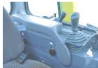
Three-stage height adjustable armrests
