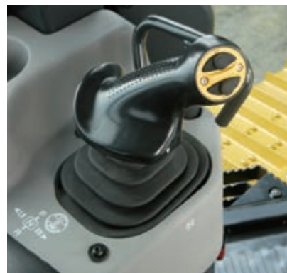
Commandes ergonomiques PCCS (Palm Command Control System)
