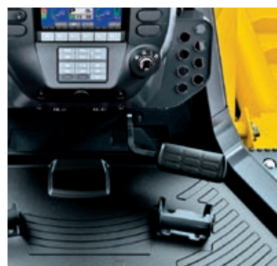
Commandes ergonomiques PCCS (Palm Command Control System)
