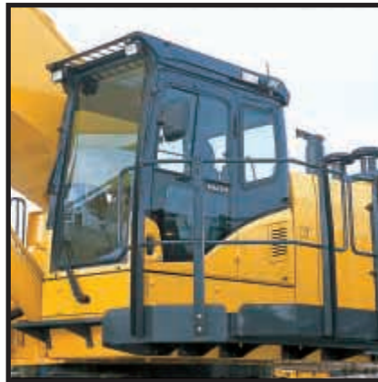
Photo shown includes Falling Object Protection System (FOPS).
