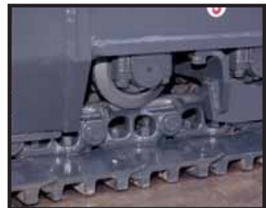
Track link with strut The PC290-7 uses track links with struts, providing superb durability
