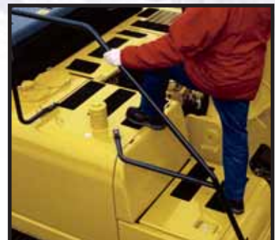
Large handrail for safe access
