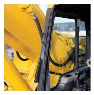
Front visibility is further improved by the use of the Komatsu patented wiper system. When not in use the wiper parks on the cab frame itself with no contact with the front window. As well as giving excellent visibility, this systems avoids the need to disconnect the wiper before lifting the front window.
