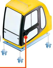
Viscous damping cab mounts ensure a quieter work environment, reducing operator fatigue whilst helping concentration.
