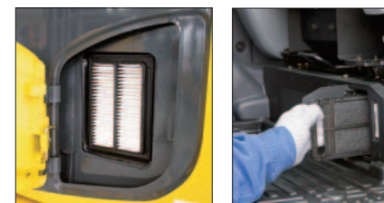
External air conditioner filter
