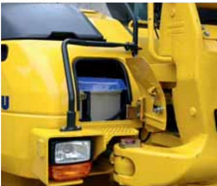
Ground level battery access
