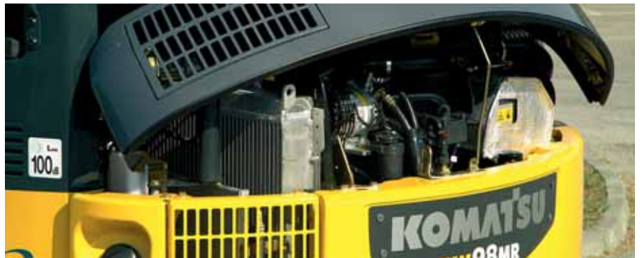
All periodic inspection points are easily accessible
