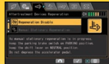
Aftertreatment device regeneration screen for the KDPF
