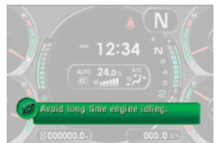
Eco guidance supports energy saving in real time
