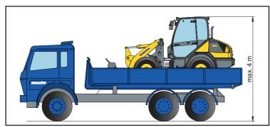
still the complete arrangement will be less than a total height of 4,0 m. Earthmoving and landscaping companies will especially welcome the rear axle-oscillation, which allows for scooping, and generally provides better stability. The rear axle-oscillation, combined with the optional 100% locking differential, makes this machine a perfect choice for gardeners.
