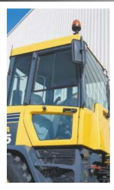
The driver's cab – driver comfort is comparable with a car Working conditions which are as pleasant as possible for the driver: easily-read, logically arranged gauges and switches, PPC hydraulic system and a multi-function lever all contribute, as do the ergonomically-designed driver's seat and the perfectlydesigned fresh air intakes, to maximum driver comfort. Attention to detail, such as the sliding window fitted as standard on the right, completes the driver-friendly picture.
