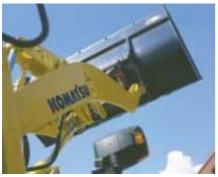
The delta boom – everything is within eyeshot The shape of the boom gives excellent vision of work attachments and tyres. Optimum working conditions, even on complicated jobs, and attachment changes which only take seconds are guaranteed.
