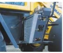
The air conditioner – For the ideal working environment The optional air conditioner, with its high-performance cooling, contributes substantially to the driver's feeling of well-being, and thus to a high rate of productivity. Thanks to its carefully designed siting on the right-hand side of the frame, it can be swung out as a complete unit for purposes of maintenance.
