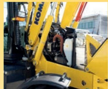
Daily maintenance is enhanced thanks to the double position front opening and the check point position easily accessible on the left side
